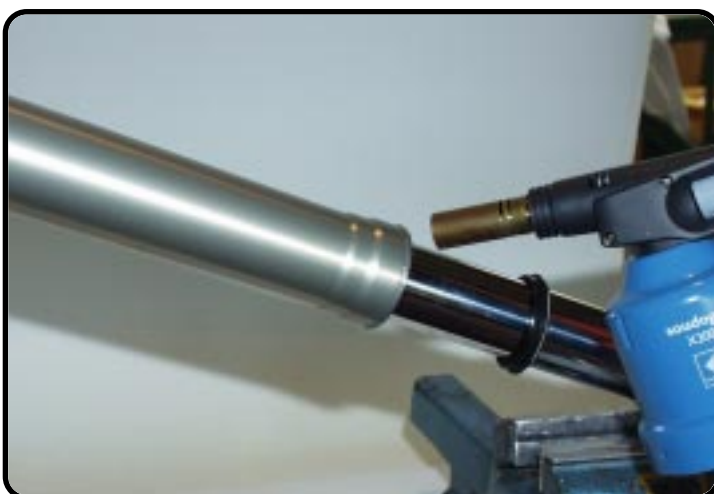
Heat the outer-tube near the oilseal. (not too hot)
