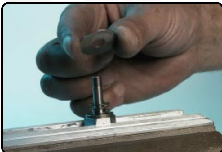
Remove check-valve shims.
