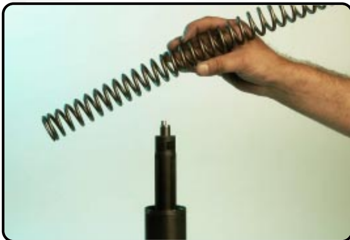
Remove the spring.
