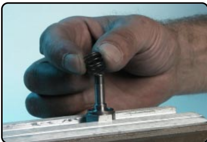
Remove spring check-valve.
