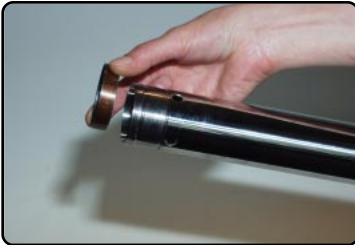
Remove DU-bush outer-tube.
