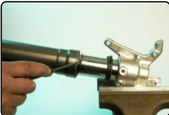
Disassemble the circlip.
