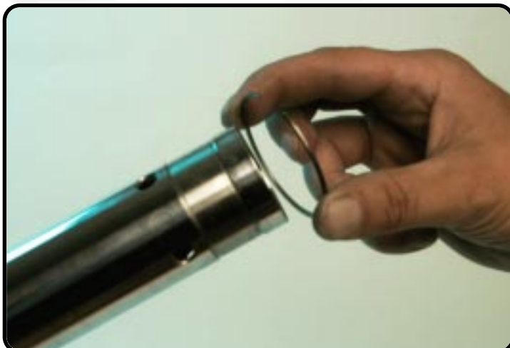
Remove the circlip.
