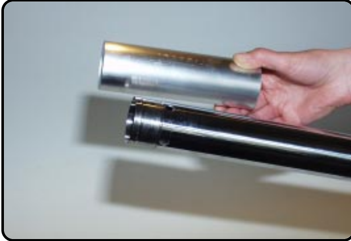
Remove DU-bush inner-tube.
